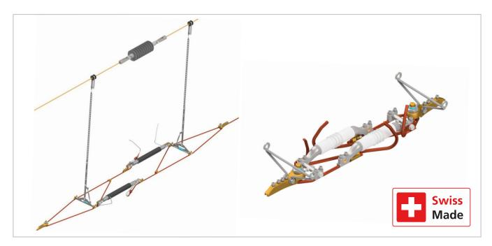
This innovative section insulator has been newly developed by Kummler+ Matter. The runners consist of copper contact wire (the contact wire of the 25/15 kV models is additionally consisting of a very abrasion-resistant it very simple to install the complete copper-magnesium alloy). Thanks to this new design, the section insulator stays flat throughout the full length. This allows the pantograph to travel smoothly across the entire length of
